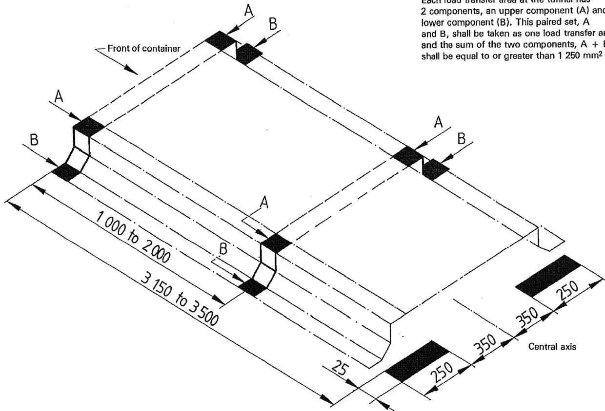
Each load transfer area at the tunnel has 2 components, an upper component (A) and a lower component (B). This paired set, A and B, shall be taken as one load transfer area and the sum of the two components, A + B, shall be equal to or greater than 1 250 mm<sup>2</sup>
